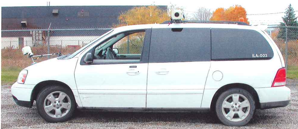
A van mounted with front and side cameras was used to photograph streets and buildings throughout Clark County.
