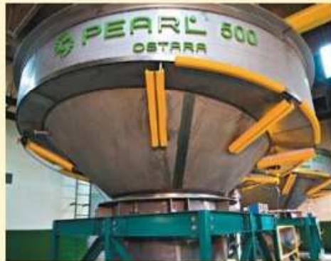
Removing phosphorous from wastewater stream - 21
